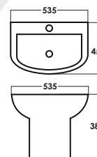
SRTWB5400 D: L535xW455xH385mm (Included Fixing Bolt)
